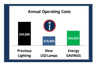
**Results** By reducing the fixture wattage from 130 to 70, the annual energy savings is 254,710 kWh, producing an electricity savings of \$30,820 per year. Over the life of the LEDs the energy savings will be approximately \$246,560. In addition to producing a Net Zero Cost of Lighting, the project also earned a \$63,704 rebate from the energy provider ConEdison.
